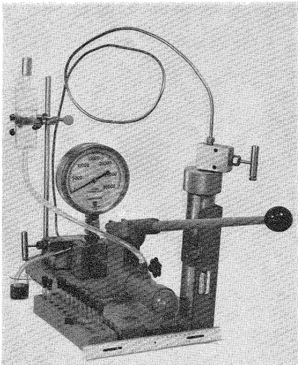
Fig. 2. High pressure vessel connected by semi-flexible steel tubing to hydraulic pump and Bourdon gauge. A rack of small culture tubes with piston stoppers is shown in foreground. ( $1/10$  natural size).
